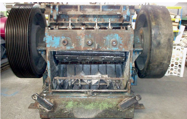
A granulator SMS 80/120 before refurbishment
