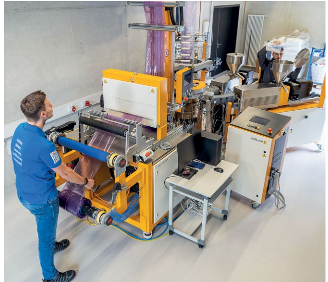
Blown film line at SKZ (Photo: Luca Hoffmannbeck, SKZ)
