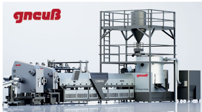
OMNI 200 Recycling System with 3C Rotary Feeder, MRS extruder, water ring pump vacuum system, twin RSFgenius screen changers and pelletising line
