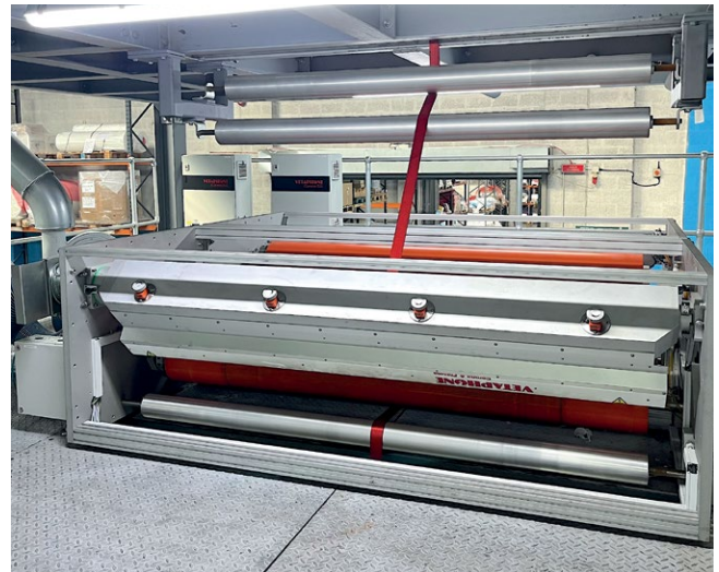
Vetaphone 1920mm VE2C-B stations are fitted to the latest Hosokawa Alpine blown film extruder at Tech Folien
